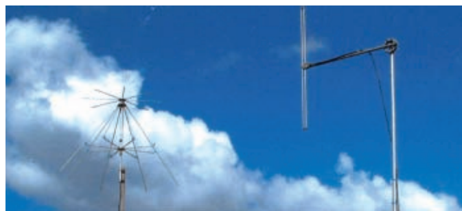
Fig. 2: The Antennas used by M3DPQ/P included a folded dipole and an interesting discone antenna, possibly made by the well known J-Beam company, once world famous for Amateur Radio antennas.
