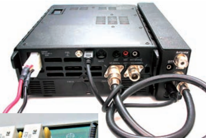
● Fig. 2: The cables at the rear of the rig and a.t.u. follow the layout shown in the manual.
