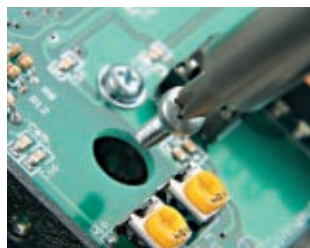
Fig. 1: Similar holes in each corner of the p.c.b. allow the AT-897 to be bolted to the side of the Yaesu FT-897 rig.
