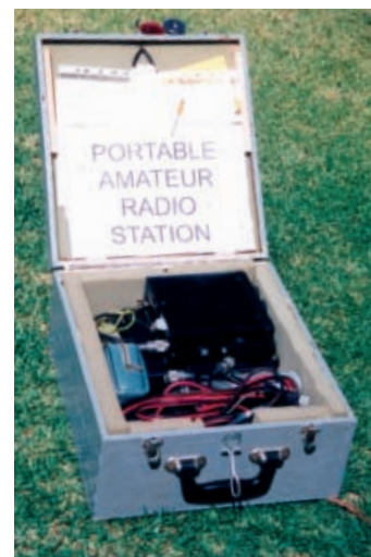
● Fig. 1: Steve's portable station on a box, the IC-706 and a.t.u. plus battery all fit into an easy-to-carry box.
