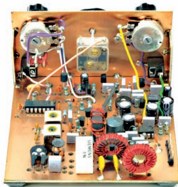
Fig. 4: Rear view of the receiver. This is built using a small printed circuit board (p.c.b.) front panel, which is soldered directly to the main printed circuit board itself. All are part of the standard kit (See information panel).
