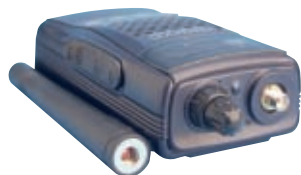
● The TH-K2E's 144MHz 'Rubber Duck' antenna is provided with an SMA type connector (see text).
